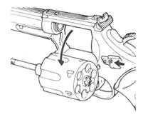
**1.** Push the latch forward, then turn out the cylinder, as shown.
