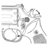
5. After exhausting the 6 rounds, pull out the cylinder and use the extracter rod to remove the shells.
