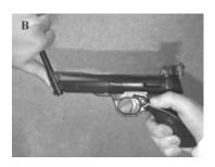
NB Never allow the barrel to spring back before the sear is engaged, nor pull the trigger until the barrel is returned and secured in its firing position.
