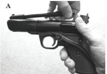
To cock the pistol hold it firmly by the grip in the right hand then with the right thumb depress the barrel as illustrated at A. Lift the barrel catch with the left hand to take up the free movement then turn the hand over so that the back of the hand is towards the body. Grip the barrel firmly then rotate it until the sear is heard and felt to engage. Keep the finger of the right hand clear of the trigger whilst cocking the pistol.
