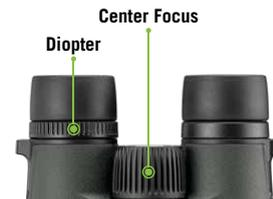
1. **Adjust the Center Focus** – Start by closing your right eye or covering the right objective lens with your hand. Look through the left barrel and adjust the center focus wheel until the image is in focus. Leave the center focus in position as you adjust the diopter.
