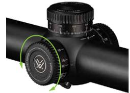
Dial the Parallax Adjustment Knob until the target image is as sharp as possible. The yardage numbers on the knob should be used as general reference points only. Check for parallax error by moving your head up, down, left, and right without influencing the gun. The parallax is correct if there is no apparent shift between the reticle and the target image. If you notice any shift, adjust the Parallax Adjustment Knob slightly until all shift is eliminated.
