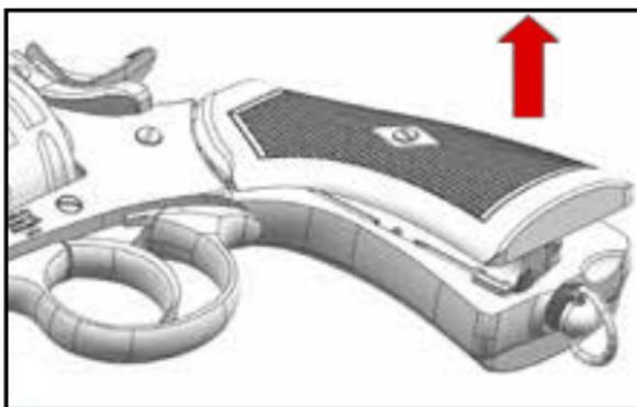
To load the CO<sub>2</sub> capsule first lift the left hand pistol grip
