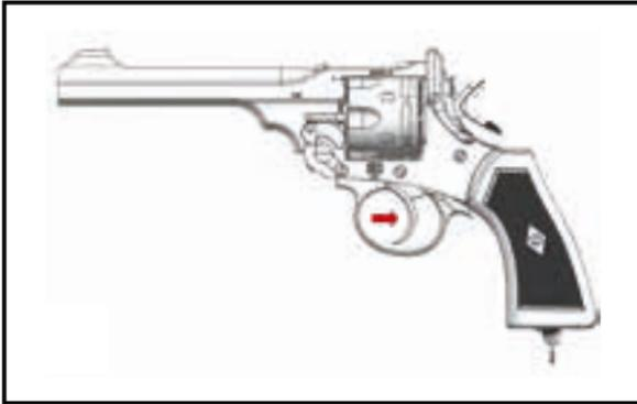
Alternatively double action for rapid fire pull back the trigger, the cylinder will rotate and the gun will fire.
