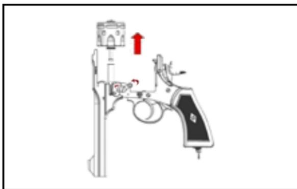
The cylinder cam can then be rotated clockwise and the cylinder can be removed from the frame. Reassemble in the reverse order
