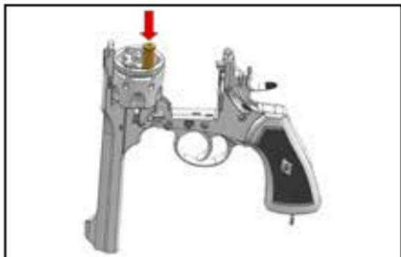
Place loaded cartridges into each chamber of the cylinder.
