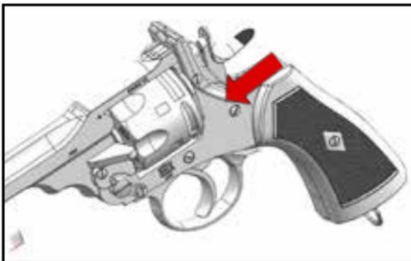
Push the barrel catch forward to open the breech
