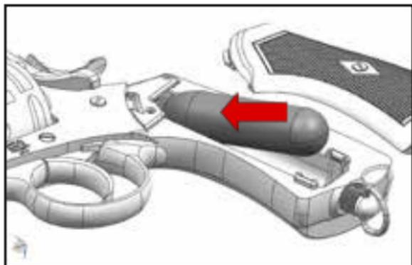
Load the CO<sub>2</sub> capsule into the CO<sub>2</sub> compartment
