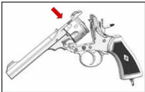
When all chambers are loaded close the barrel making sure that the barrel catch is in the fully locked position
