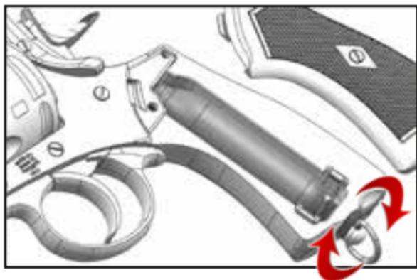
Turn the lanyard swivel clockwise to charge the CO<sub>2</sub> capsule
