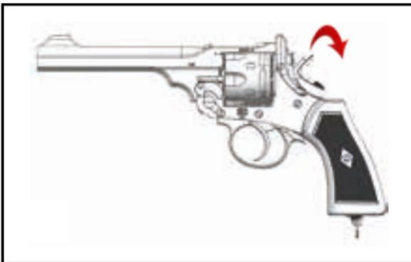
The Webley MK VI Revolver can be operated single action with the gun in the firing position, pull back the hammer using your thumb, the hammer will then lock in the rear position. The gun can now be fired with a lighter trigger pull for target shooting.
