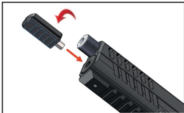
Remove the end cap and Load the CO<sub>2</sub> capsule into the CO<sub>2</sub> compartment.
