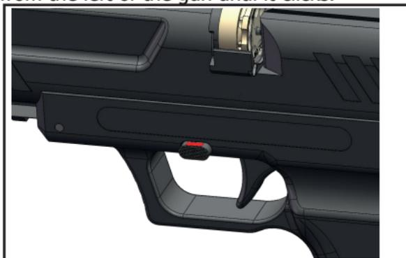
Push the bolt fully forward, press the Safety Catch fully to left until the red fire indicator is visible when ready to fire.
