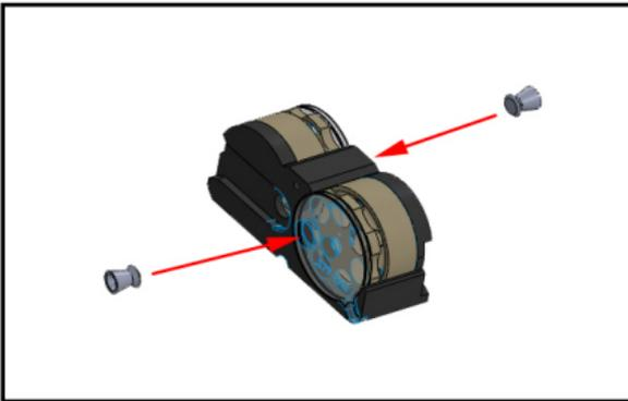
Push pellet's nose first into the transparent faceplate on either side of the Magazine, rotate the central cylinder anti-clockwise to the next empty chamber, push in the next pellet. Repeat for the amount of shots required. Repeat on the reverse side of the Magazine.
