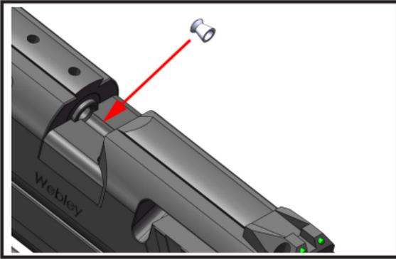
Pull the bolt to its rear position, fit the Single Shot Tray as shown.
