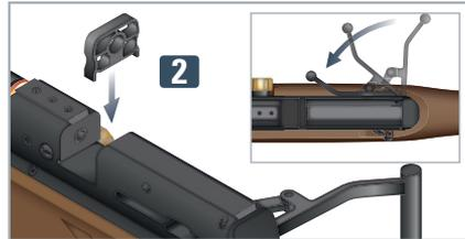
2. Insert the spacer **2** as shown and close the cocking lever.
