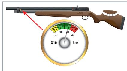
3. Watch the gauge on the air rifle and charging equipment. We recommend to fill the tank with a pressure of 200 bar. **Do not exceed a filling pressure of 200 bar!**
