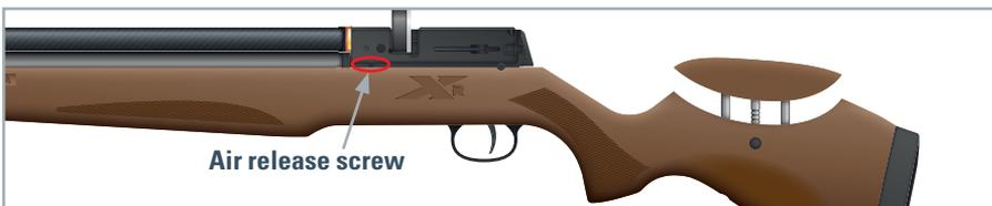
**Note:** Ideally, there is always some pressure in the compressed air cylinder to protect the seal and prepare it for the next filling process. If you really need to empty the compressed air cylinder completely, loosen the drain screw slightly until you can hear the air escaping. Never unscrew the
