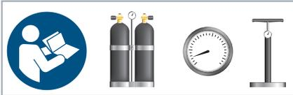
1. Read all instructions about your charging equipment. **Please note that your charging equipment must include a pressure gauge (manometer)!** Ensure that all connections are free from dirt.
