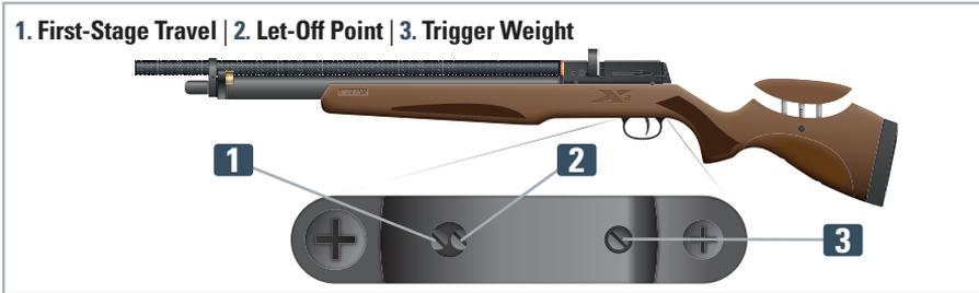
**Note:** Use a slot screw driver to adjust the trigger.
