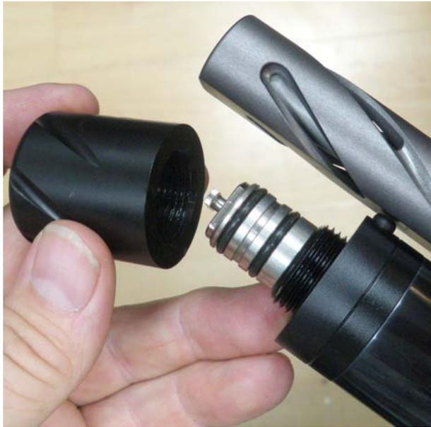
*This achieved by unscrewing the cover in an anti-clockwise direction.*
