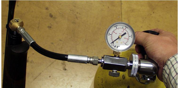
Once the filling pressure has been reached, close the valve on the bottle or stop pumping, open the bleed valve on the filling kit (to vent the hose, if you do not vent the hose you will not be able to remove the female from the rifle). Now the female connector can be removed from the rifle and end cap (E483BK) can be replaced over the male connector ensuring not to over-tighten.
