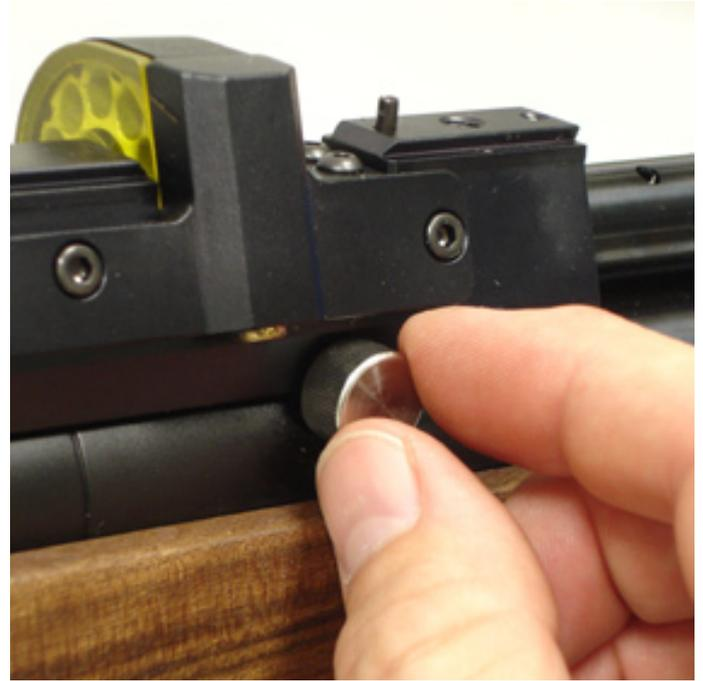
On the left hand side of the rifle is an indicator to help select your most common power settings + = High. - = Low. The marks do not indicate a particular power as this would change depending on the pellets used. The engraving maybe marked the other way round to the image below. This is normal and for manufacturing purposes.
