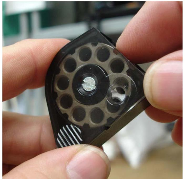
Hold the magazine and drop a pellet into the chamber. Manually index to the next empty chamber and repeat until the magazine is full. Finally line up the red dot on the pellet carrier with the 'V' notch on the clear magazine cover.
