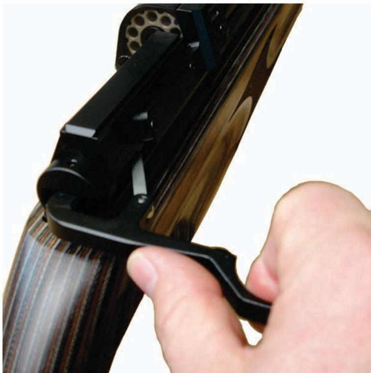
**Note !** It is very important that the cocking lever is pulled back to the correct position. In one positive motion. The magazine indexes to the next pellet position as the bolt is retracted and it is possible for a partial index if the lever is not pulled back fully.
