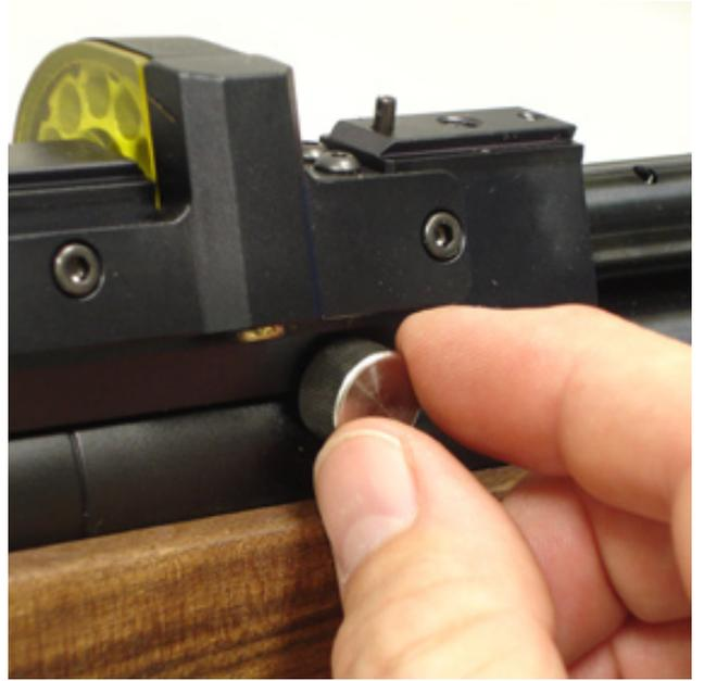
On the left hand side of the rifle is a indicator to help select your most common power settings + = High. - = Low. The marks do not indicate a particular power as this would change depending on the pellets used.
