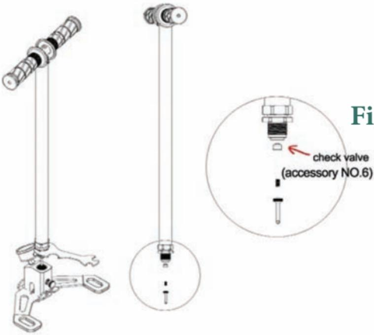
Using the spanner wrench, open the check valve in the base plate. Clean or replace the check valve.
