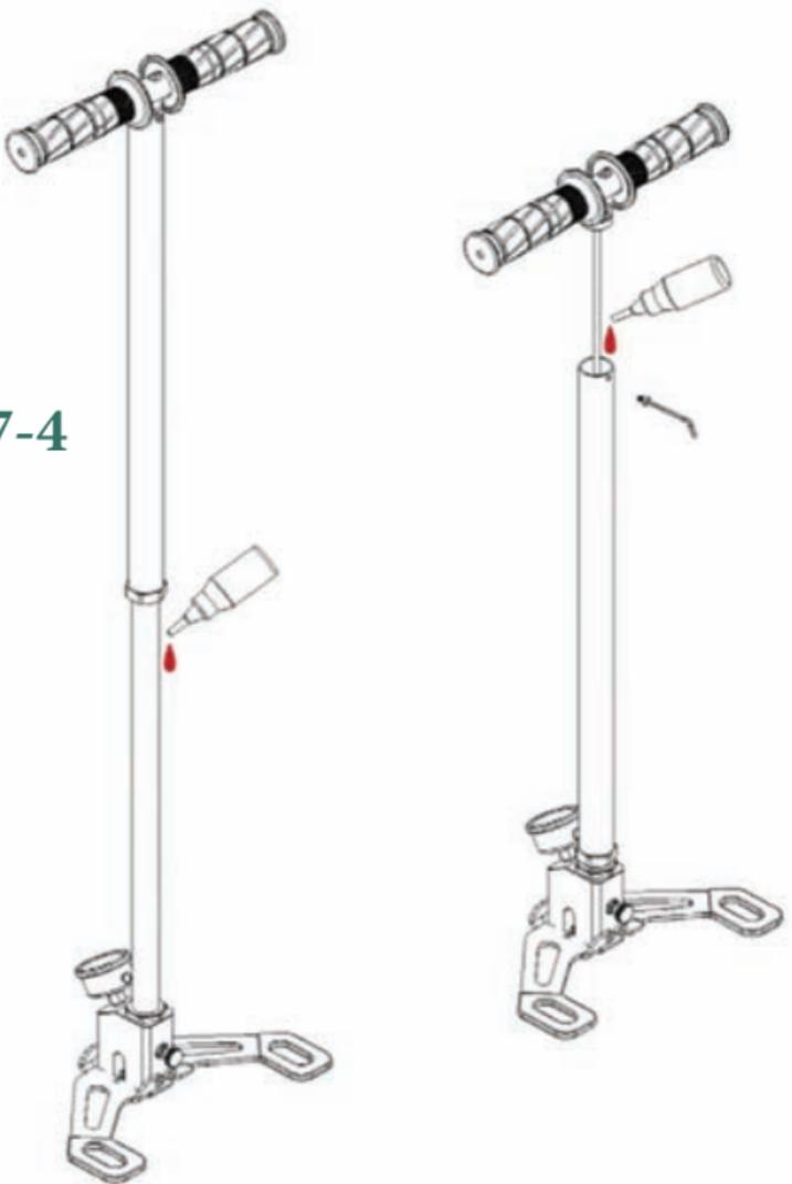
Lubricate pump with silicone oil as shown.
