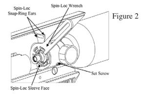
NOTE: If you have a Quick-Detach Air Tank, without the gauge and refill fitting, tighten the set screw to keep the Spin-Lock Sleeve from turning. Then screw in your Quick-Detach Tank as you normally do in a standard frame.
