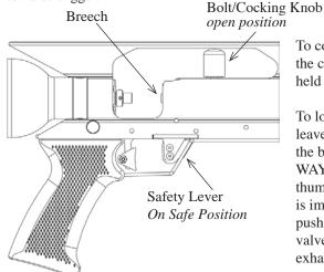
To cock the rifle, push forward on the cocking knob until the bolt is held in the open position.
