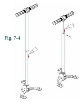
Lubricate pump with silicone oil as shown.
