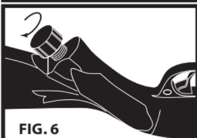
**WARNING:** Be sure the muzzle is pointed in a safe direction when puncturing a CO2 cylinder. In the event that a seal temporarily leaks while a CO2 cylinder is being punctured, the CO2 gas may escape through the barrel. If ammunition is jammed in the barrel from prior shooting, this could result in a projectile being shot.
