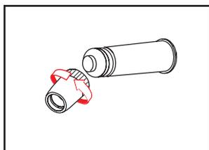
Unscrew the pellet compartment from the cartridge, by turning it counterclockwise.
