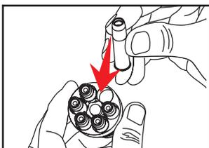
Place the cartridges in the speedloader.
