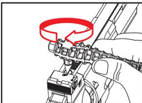
Turn clockwise to fasten the screw.
