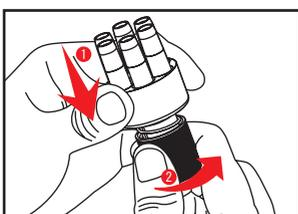
Push down the speedloader and turn right to lock the cartridges.
