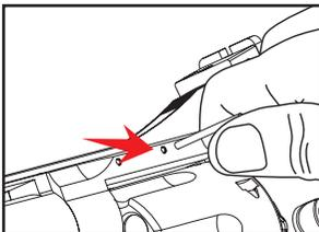
Put rear sight and spring back and insert the spindle.
