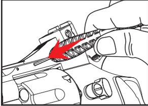
Use tool to pin out the spindle from the gun's left side and take out the aiming hole.
