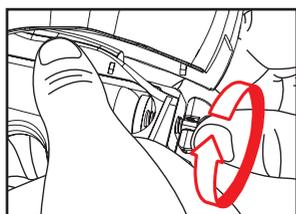
Turn the lock system clockwise to activate the CO<sub>2</sub> capsule. Remount the CO<sub>2</sub> handle cover.
