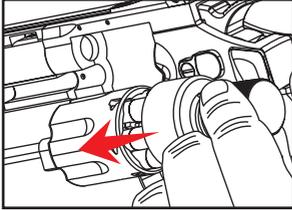
Insert speedloader into the cylinder. Push until cartridges are released into the cylinder.
