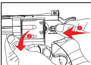
Use right thumb pushing safety to "Open" then use left hand to push out the cylinder.
