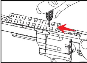
Put in tactical rail. Use tool to fasten screws and fix tactical rail.
