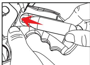
Load the CO<sub>2</sub> capsule into the CO<sub>2</sub> compartment.
