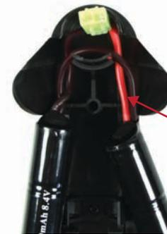
**Step 4.** To attach the stock pad you will need to reverse the steps. Press in on the top tab and pivot inward. Gently press on and make sure not to damage any parts. Please notice the wires going through the slots in the stock pad for correct install.
