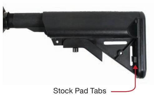
**Step 1.** Gently press inward the two tabs on the Stock Pad. About 2mm and should be clear. Pull back on the stock pad to remove.
