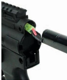
**Step 2.** To insert the 9.6v stick battery first straighten the wires if needed. Notice the wire along side the row of battery cells. Keep the wire or spine to the bottom left or right as you slide the battery into the gun.
