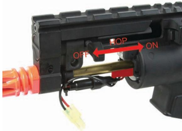
**Step 2.** To adjust the hop up unit you will have to slide the bar back or forth. Adding UP will add more hop up effect and turning OFF will turn the hop up unit off. Once you find the best setting you can install the hand guard.
