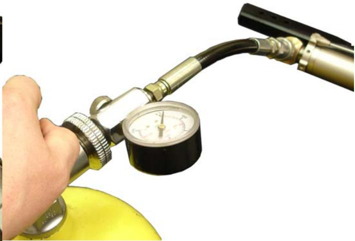
Once the connector is exposed the female part of the filling kit can be place on the male and press all the way on making sure that the 'O' rings on the male part are covered.
