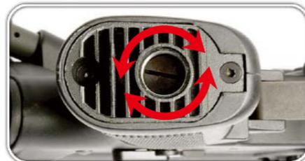
The motor adjustable screw is at the bottom of the grip. Use a screwdriver to adjust.
