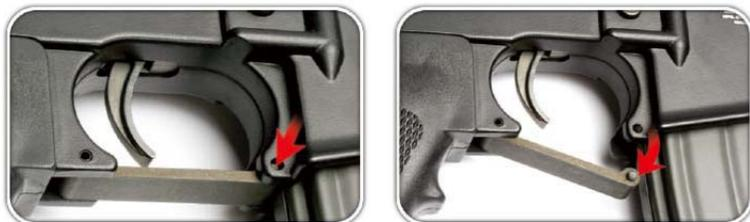
Depress the trigger guard plunger with a proper tool and open the trigger guard.
