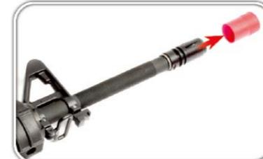
Remove the protective cap only when you are ready for firing the gun.
