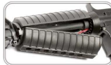
Pull the slip ring and hold. Remove the lower handguard.
