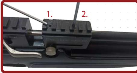
Dissamble the assemble screw of the receiver.(screw1)
