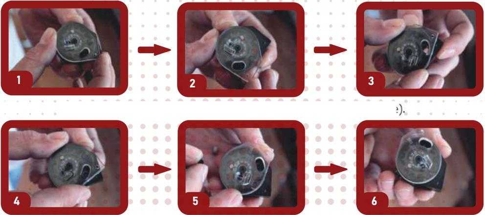
Once the glass cover hits are last point, prevent the pushing force of the spring and switch the Pellet to first bed(see picture 4).Once the first pellet prevents the rotation of the inner turret, move the glass cover on the contrary direction and fill the turret.
