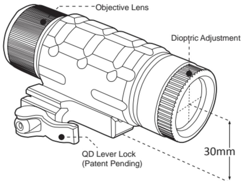
Medium Profile Configuration with Riser & Mounting Deck
