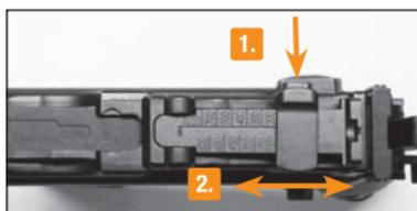
To adjust sights (elevation only), press and hold button, then slide forward or backward
