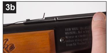
4) Align the rear anchor hole in the mount over the hole for the stock screw at the top rear of the receiver.
