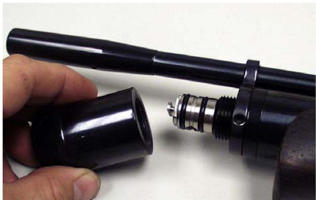
*This is achieved by unscrewing the cover in an anti-clockwise direction.*
