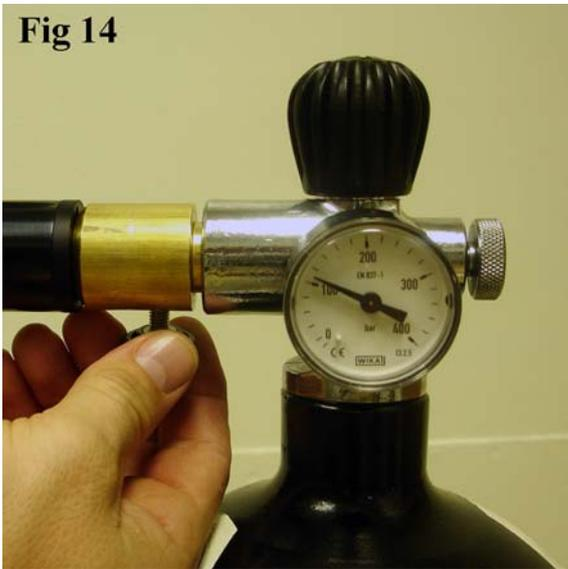
Once the desired pressure is reached close the main valve on the filling bottle or stop pumping. Open the bleed valve on the adaptor, this will vent the trapped air in the hose and allow the cylinder to be unscrewed from the adaptor. If you don't vent the adaptor, air trapped in the hoses makes removing the cylinder from the filling kit very difficult and may cause damage to the adaptor seals.
