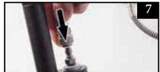
**! CAUTION:** Always check and make sure the collar on the female quick disconnect is in the forward position and secure on the male fitting you are connecting it to. It is recommended that you check the connection by attempting to pull the female and male ends apart while the collar on the female fitting is in the forward position.
