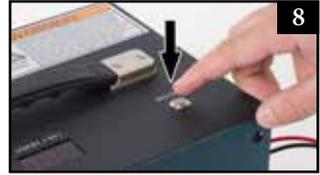
9) Once the pre-set fill pressure is reached, the compressor will stop.
