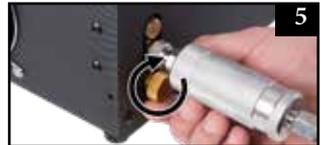
6) On the underside of the unit, locate the "Moisture Release Valve" and turn clockwise until tight.
