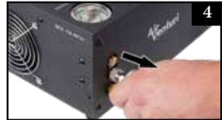
**! CAUTION:** Always check and make sure the collar on the female quick disconnect is in the forward position and secure on the male fitting you are connecting it to. It is recommended that you check the connection by attempting to pull the female and male ends apart while the collar on the female fitting is in the forward position.
