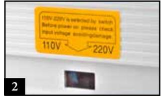
**3)** Locate the adjustment window on the power converter. Using an allen key, move the switch to the desired input power setting. If the switch is on the left, 110V is selected. If the switch is on the right, 220V is selected.
