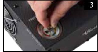
**! WARNING** DO NOT OVERFILL AIR CYLINDERS OR AIR GUN TANKS, AS THIS CAN CAUSE SERIOUS INJURY OR DEATH. NEVER SET THE OUTPUT PRESSURE/AUTO SHUT OFF ABOVE 4500 PSI (310 BAR).
