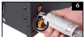
7) On the underside of the unit, locate the "Moisture Release Valve" and turn clockwise until tight to close it.
