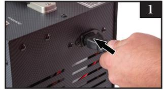
2) Plug the 110V three prong connector into your wall outlet (fig. 2). Once plugged in, the fan on the power converter will turn on. The compressor fans and **LOAD** gauge will not come on yet.
