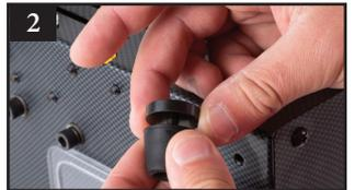
3) Replace each foot with the extension by turning them clockwise (fig. 3a).until they are tight against the bottom of the unit. (fig. 3b).
