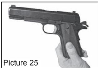
**WARNING!** If the hammer does **NOT** remain cocked when the grip is not depressed, the air pistol is **NOT** safe to use. It must **NOT** be used until you have it inspected and corrected. Call Remington's Consumer Service at 1-800-243-9700. Discharging an air pistol which does not function properly may lead to property damage, personal injury and/or death.
