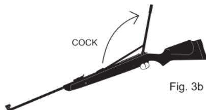
**(SIDE-LEVER)** — Firmly grasp the air rifle in a manner which will not interfere with the cocking lever. Pull the side lever toward butt of the gun until it comes to a solid stop (See Fig. 3b). This action will cock the gun and open the breech.
