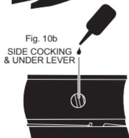
**⚠ CAUTION:** OILS THAT CONTAIN ACID OR RESIN CAN DAMAGE THE BREECH SEAL, COMPRESSION SEAL, AND POSSIBLY THE FINISH OF THE STOCK.
