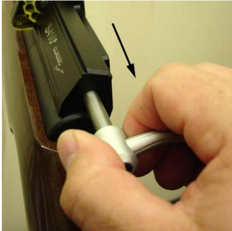
Note ! It is very important that the loading bolt is pulled back to the correct position in one positive motion. The magazine indexes to the next pellet position as the bolt is retracted and it is possible for a partial index if the bolt is not pulled back fully.
