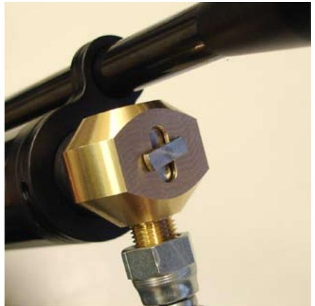
If the rifle is empty the mechanism will need to be cocked to allow the firing valve to close. If the rifle is not cocked when the bottle is opened or the pump used, the air will pass the valve and exhaust through the barrel.
