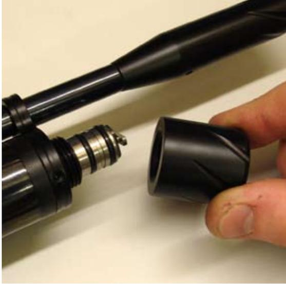
Once the connector is exposed the female part of the filling kit can be placed on the male and pressed all the way on, making sure that the 'O' rings on the male part are covered.
