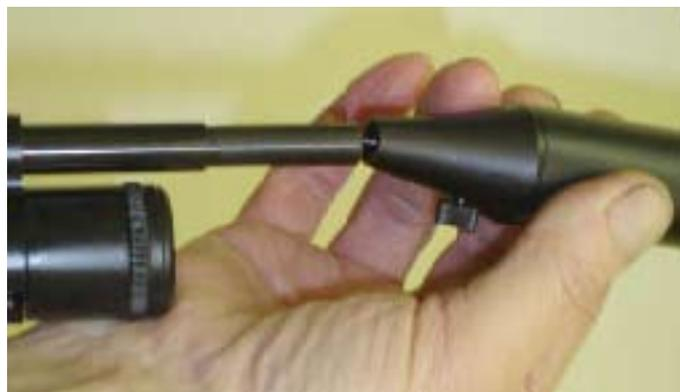
To remove the rear stock from the rifle, the fixing wheel at the back of the stock (KS460) must be turned anti-clockwise. When this is loosened fully the rear stock will come away from the fore-end.
