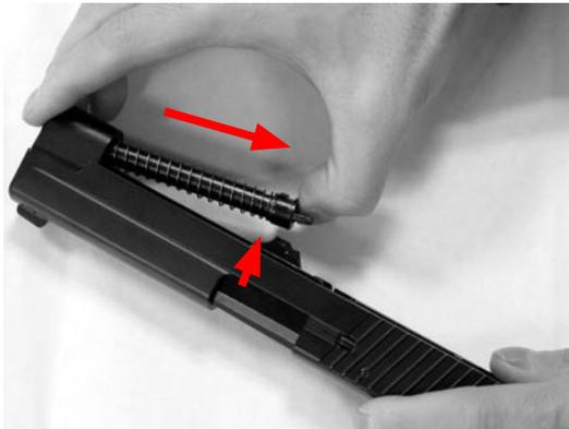
REMOVE THE RECOIL SPRING GUIDE AND SPRING.
