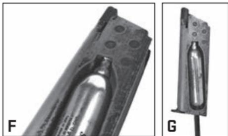
NOTE: Slight seepage may occur when tightening canister as the gas pin punctures CO<sub>2</sub> cylinder.
