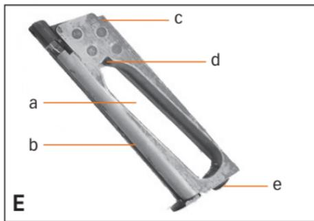
2. Using the 1/4" allen wrench provided with the gun, loosen the cartridge screw at the bottom of the magazine housing by turning counterclockwise.
