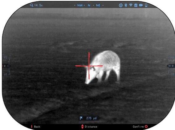
Change distance value using the Keypad buttons
