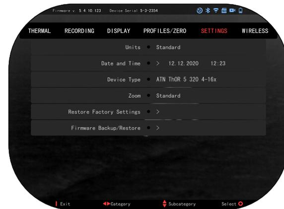
**DEVICE TYPE** — to make all features work correctly you need to choose the type of lens you have. (Example: 3x stands for 3-12 and 5x stands for 5-20).
