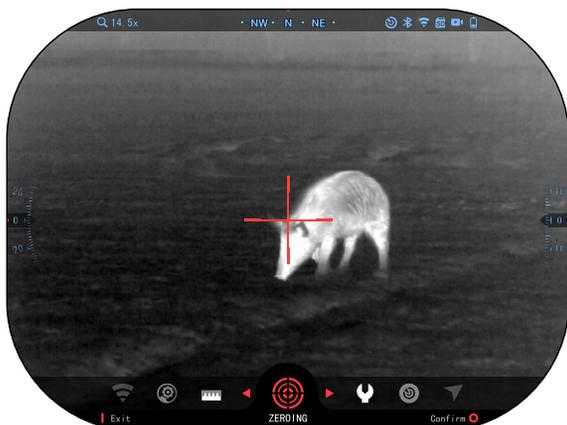
a cross hair reticle. While keeping the gun as steady as possible, fire a round. Use the key pad to move the Red cross hair to the point of impact. While keeping the White crosshair in the same place you where aiming. Once you have placed the Red crosshair on the POI, press the OK button. A dialogue box will appear with options. Select Save & Exit.
