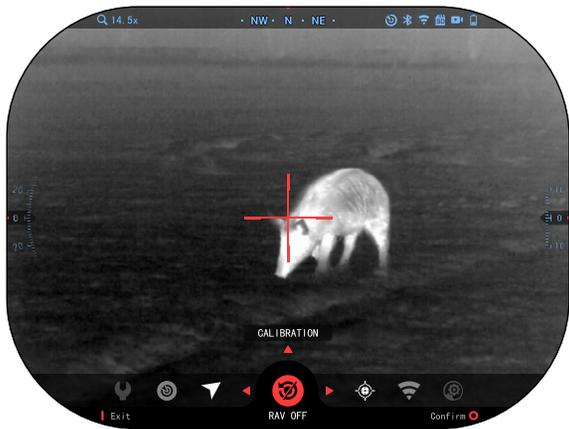
When a shot is fired and your scope experiences recoil (some airguns may not provide enough recoil for RAV to be activated). The scope will record video prior to the shot being taken, the moment of, and some time after. Exact settings may be adjusted in the System Settings.
