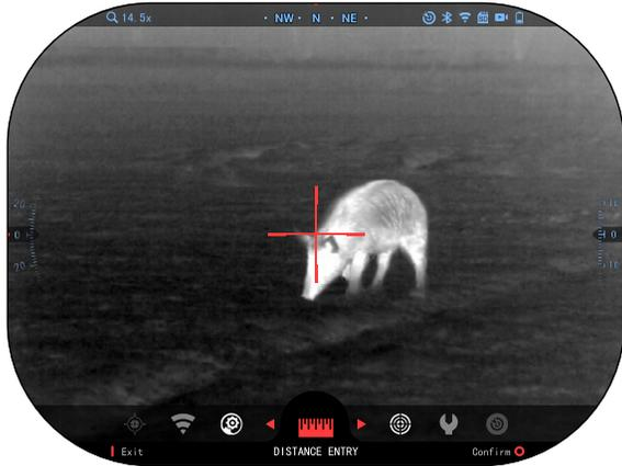
Allows you to input or correct the distance manually. Choose the Distance Entry option to launch this function.
