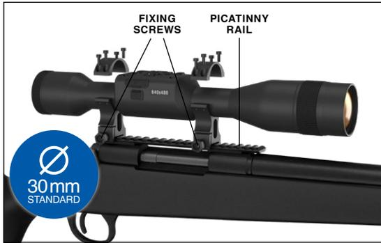
The ThOR 5 has a 3.5-inch eye relief (90 mm), and can be mounted using 30 mm mounting rings. ATN has provided two standard rings and one L shape ring. The L shape ring is for those instances when you need extra eye relief for certain rifles. First, choose your preference of rings and position and mount the bottom portions of your rings to your rail for optimal eye relief. Place
