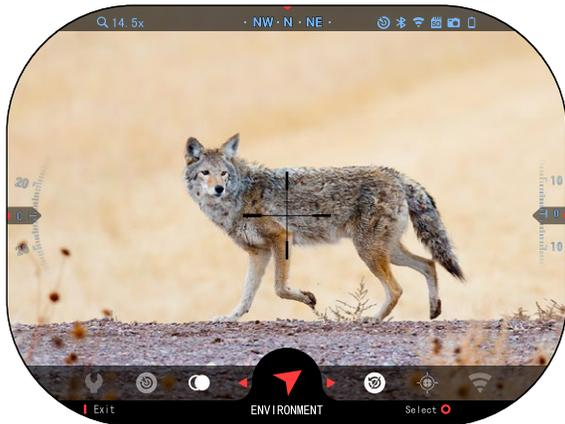
Icon. Press the OK button to enter it. Use the UP and DOWN buttons to adjust wind speed. use the RIGHT and LEFT buttons to adjust the wind direction. To adjust other environmental settings press the FUNCTION 2 button. Press the OK button to confirm your changes. Press the FUNCTION 1 button to escape the Menu.
