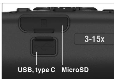
The device is equipped with a microSD Card and USB (type C) ports. You can find them under the rubber caps on the right side of the device (we marked the caps with appropriate icons).
